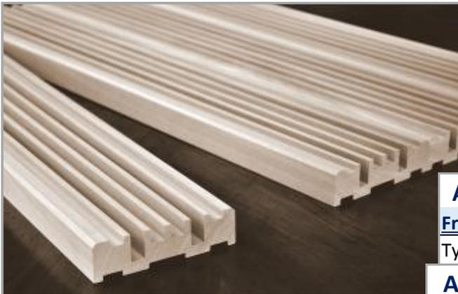
Type-LFA (optional) has rear reliefs engineered to provide additional absorption below the frequency range of the diffuser cut-off frequency. Installation mounting is by traditional screw/glue methods directly to most architectural surfaces. Additionally, plank profiles can be installed with a rear air space, slight separations, and a glass or polyester fiber back-layer for increased low frequency absorption.
